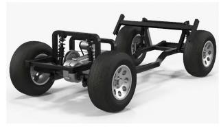
Whether in their assembled or unassembled form, rolling chassis may also be accompanied by other components and subassemblies such as batteries, bumpers, wheels/tires, cowlings, fenders, grills, kick plates, steering column and steering wheel assemblies, dash assemblies, seat assemblies, pedal assemblies, brake assemblies, canopy or roof assemblies,
